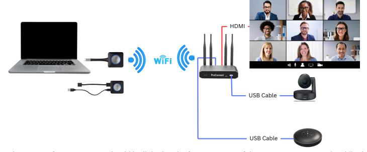
The USB conference camera should be linked to the front USB port of the ProConnect Base Unit, while the USB conference omnidirectional microphone and speaker should be connected to the rear USB port. Connect the HDMI output of the ProConnect Base Unit to a large display or projector. Note that if the conference camera incorporates audio, prioritize connecting the USB conference omnidirectional microphone and speaker to the rear USB port of the ProConnect Base Unit for optimal audio quality.
